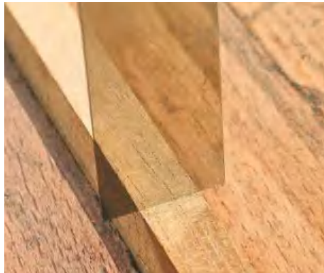
▲ Pic.6 ... but getting the chisel square both ways makes it look transparent
